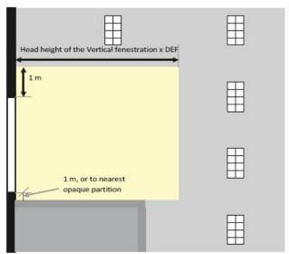
**Daylight Extension Factor (DEF):** factor to manually calculate the daylight area on floor plates. It is to be multiplied by the head height of windows. It is dependent on orientation and glazing VLT, shading devices adjacent to it and building location.
