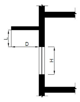
**Projection factor, side fin:** It is the ratio of the horizontal depth of the external shading projection to the distance from the window
